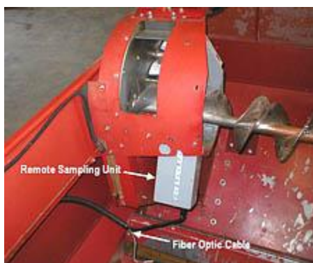
Fig. 1. Remote sampling device (with cables) mounted to the exit auger in the bulk tank of a Case-IH model 1660 combine harvester.
